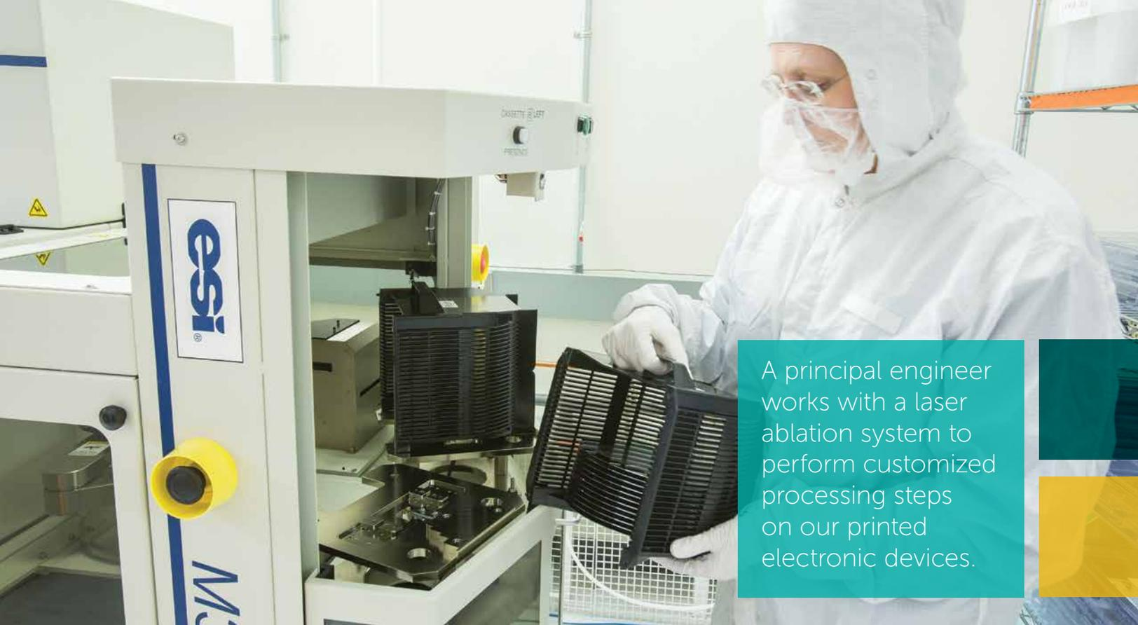
A principal engineer works with a laser ablation system to perform customized processing steps on our printed electronic devices.
