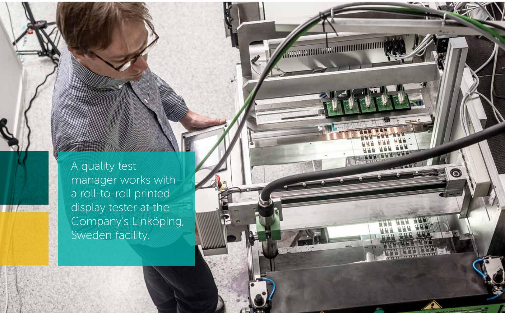
A quality test manager works with a roll-to-roll printed display tester at the Company's Linköping, Sweden facility.
