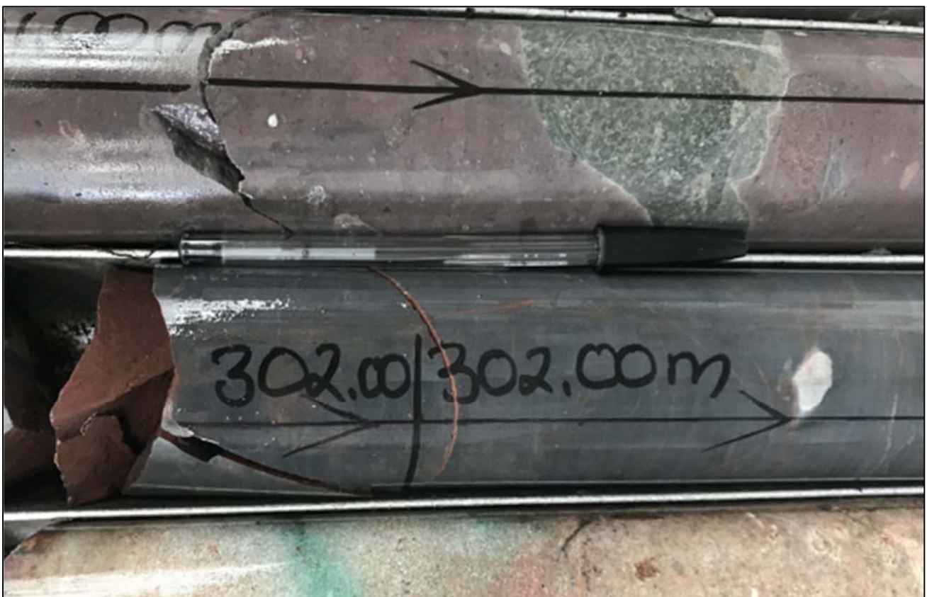
Figure 8: Maroon diamictite, siltstone with disseminated chalcocite drilled in the southern edge of Kakula West.
